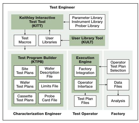
Figure 3. KTE software architecture
